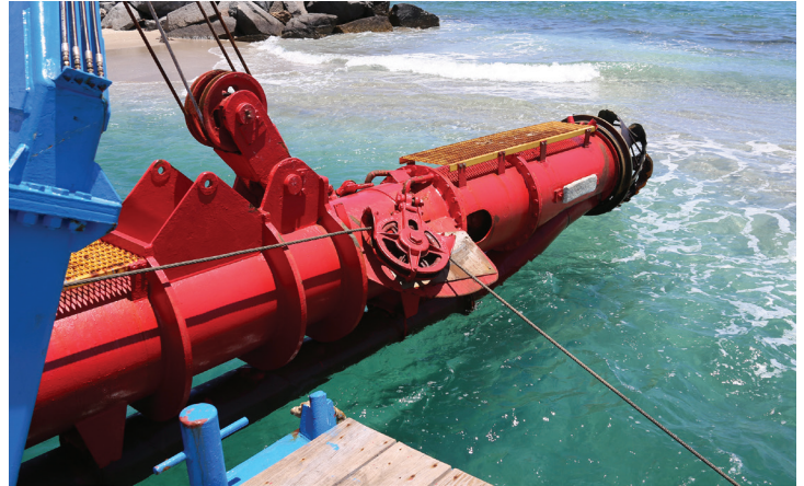
Ellicott winch-controlled dredge arm at Hillsboro Inlet
