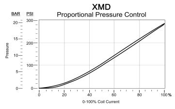
Example showing the **PRDL** pressure control valve combined with XMD precision.
