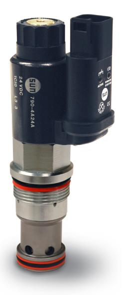
Sun's pilot operated, high capacity, electroproportional throttle valve expands our growing family of electrically actuated screw-in cartridges and in particular, enhances our flow control product offering. Model <u>FPHK</u> is available in 40 and 60 gpm (160, and 240 L/min) capacities.
